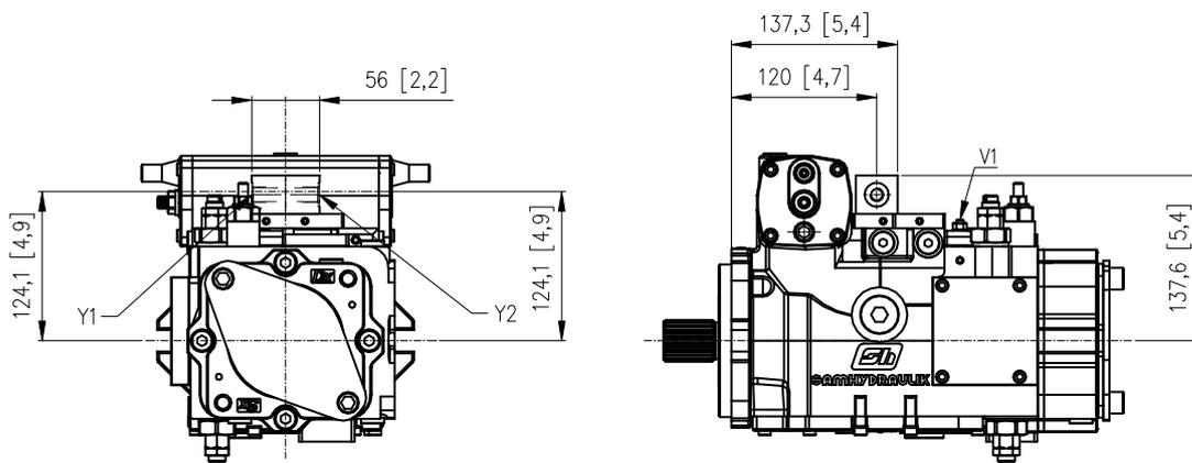
Y1-Y2: Attacchi pilotaggio comando / Control piloting pressure ports - 1/4 G (BSPP)
