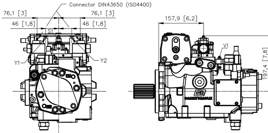
Y1-Y2: *Attacchi pilotaggio comando* / Control piloting pressure ports - 1/4 G (BSPP)
