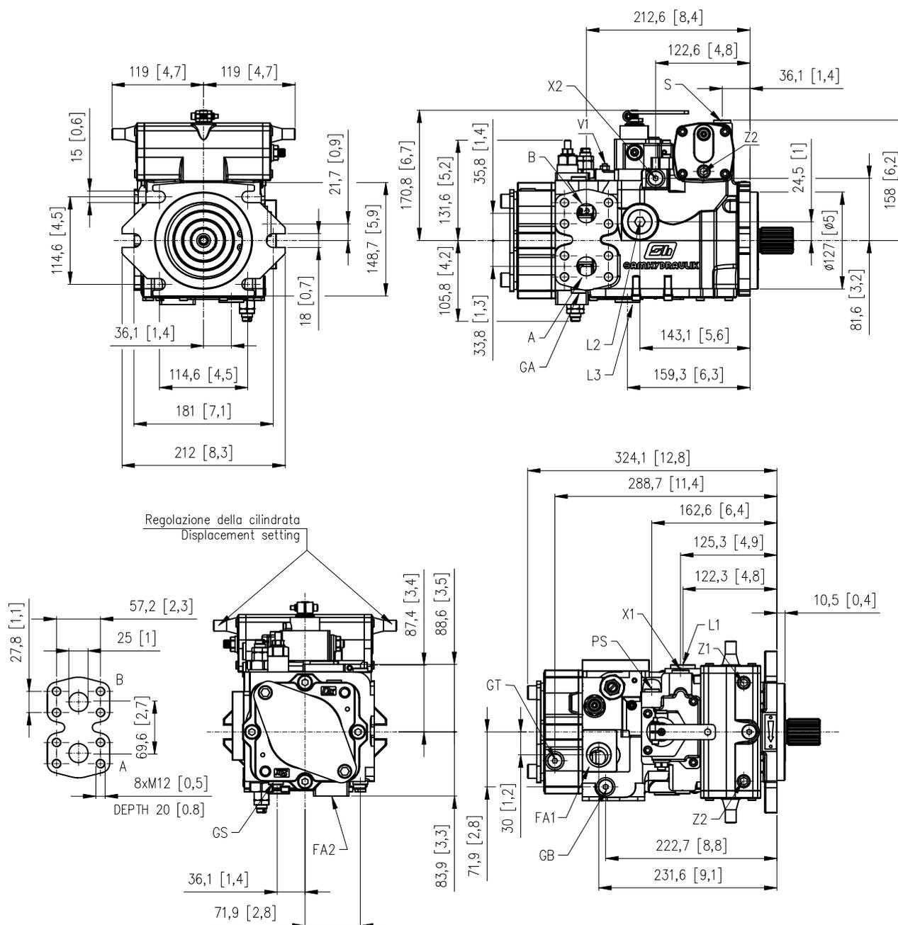
A-B: Linee in pressione / Pressure ports - 1" SAE 6000
