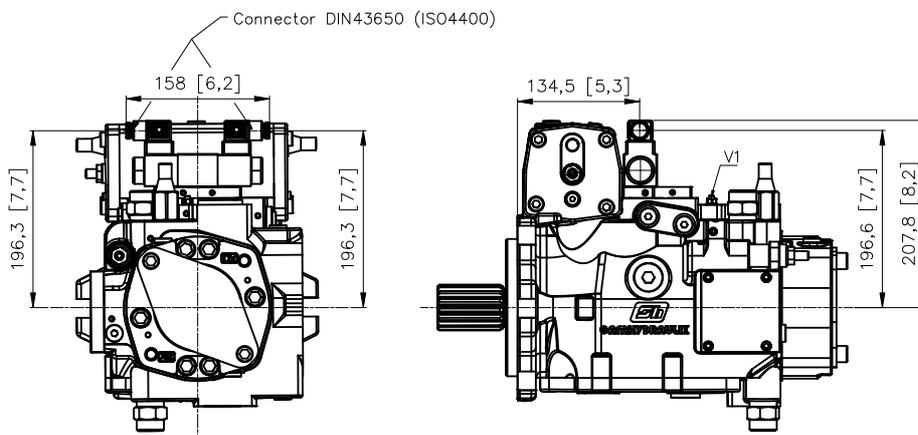
V1: Strozziatore variabile / Adjustable throttle valve
