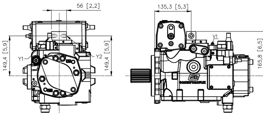
Y1-Y2: Attacchi pilotaggio comando / Control piloting pressure ports - 1/4 G (BSPP)
