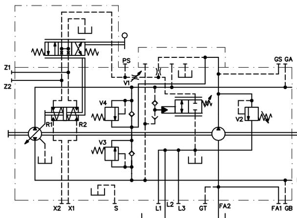
Note: The pressure compensator valve is always mounted on SH6V 130 pump and it can be combined with electric cut-off (EP) valve. For working pressure higher than 380 bar [5510 psi], the valve is locked
