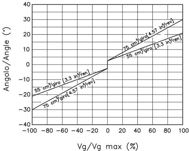
The displacement of the pump is directly proportional to the angle of the lever. The feedback system feels the position of the washplate and works automatically to compensate for a positioning error. The micro switch is built as PNP, therefore the sensor is in  $T_{low}$  when the lever is in neutral position. Any movement of the lever brings the sensor in  $T_{high}$ . The diagram below shows the relationship between angle and displacement.
