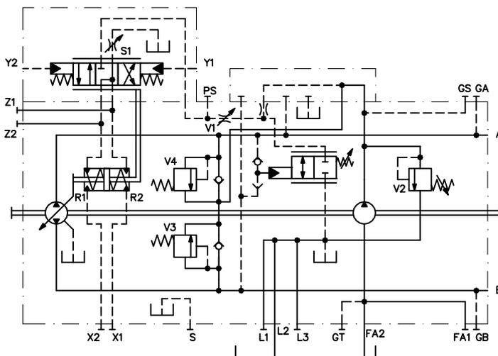
Pilot pressure = 6÷18 bar [87÷261 psi] (at ports Y1, Y2)
