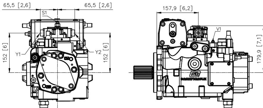
Y1-Y2: Attacchi pilotaggio comando / Control piloting pressure ports - 1/4 G (BSPP)
