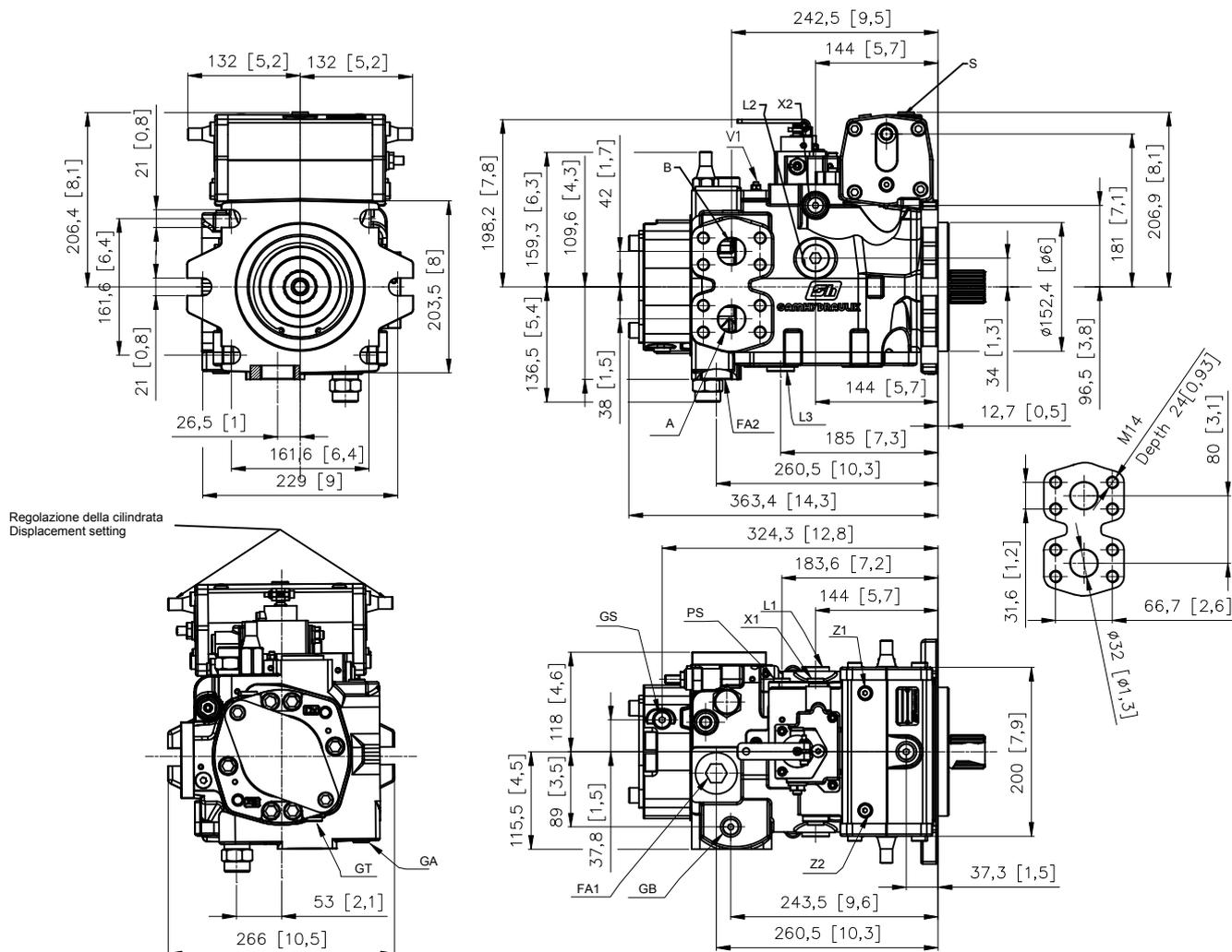
A-B: Linee in pressione / Pressure ports - 1"1/4 SAE 6000
