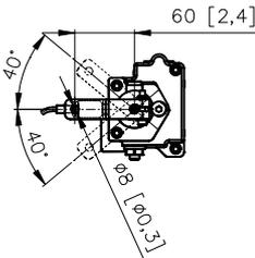
The displacement of the pump is directly proportional to the angle of the lever. The feedback system feels the position of the washplate and works automatically to compensate for a positioning error. The micro switch is built as PNP, therefore the sensor is in  $T_{low}$  when the lever is in neutral position. Any movement of the lever brings the sensor in  $T_{high}$ . The diagram below shows the relationship between angle and displacement.
