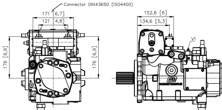
V1: Strozziatore variabile / Adjustable throttle valve
