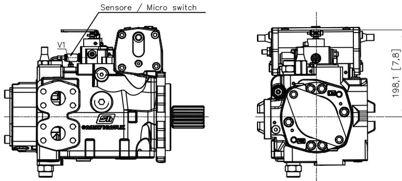
V1: Strozziatore variabile / Adjustable throttle valve
