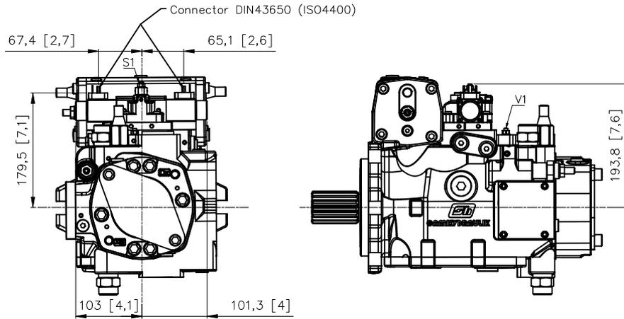
S1-V1: Strozziatore variabile / Adjustable throttle valve
